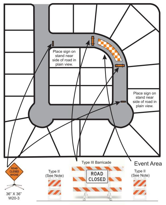
Place the Type III Barricades at the ends of the event area as specified in the permit request. Road widths greater than 30 feet shall be supplemented with Type II Barricades on either side of the Type III Barricades to prevent vehicles from passing on the sides. Remove as soon as the event is completed. Barricades and setup must be Manual on Uniform Traffic Control Devices (MUTCD) compliant. Refer to
