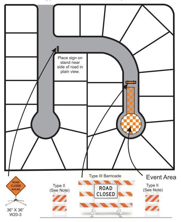
Place the Type III Barricade at the end of the event area as specified in the permit request. Road widths greater than 30 feet shall be supplemented with Type II Barricades on either side of the Type III Barricade to prevent vehicles from passing on the sides. Remove as soon as the event is completed. Barricades and setup must be Manual on Uniform Traffic Control Devices (MUTCD) compliant. Refer to
