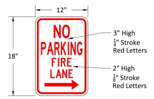
**Fire Lane Sign Characteristics:** Signs shall be engineer grade reflective sheeting on 0.80 aluminum with red lettering on a white background.
