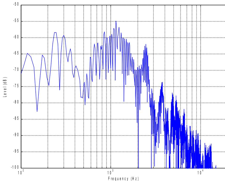
**Figure 6.3. Spectral Response of a Dull Hit**
